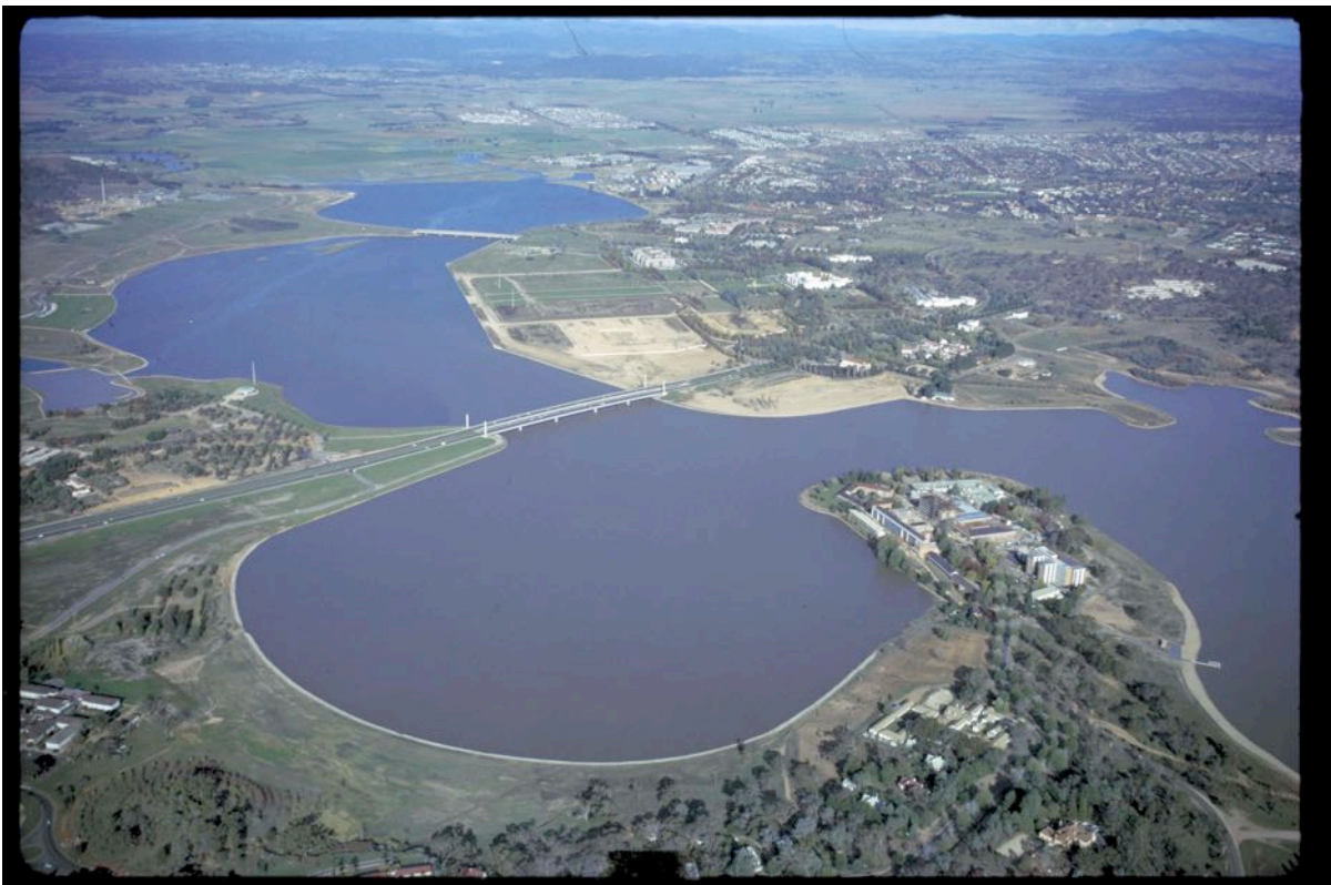
Figure 2: Image taken by Richard Clough 1964 from Black Mountain after the lake filled, showing the horseshoe shape of West Basin and the changed delineation of Central Basin with the bevelled edges to the southern shore to ensure water flow. (Image courtesy of the National Library of Australia)
