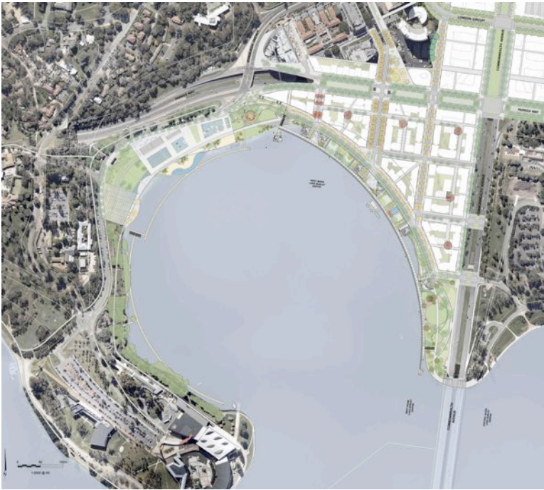
Figure 3: Proposed development at West Basin as part of the City to the Lake project that includes a total of 2. ha lake infill in the northern area and .8ha of infill at the park near Commonwealth Bridge. (image from the former ACT Land Development Authority)
